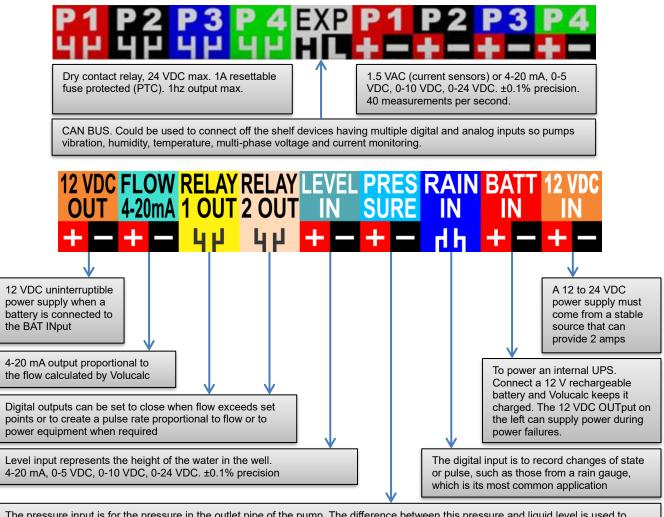
The pressure input is for the pressure in the outlet pipe of the pump. The difference between this pressure and liquid level is used to calculate the head pressure. If not used for pressure, it can be used for something else like getting flow from another flow meter. or 4-20 mA, 0-5 VDC, 0-10 VDC, 0-24 VDC. ±0.1% precision
