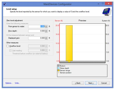
and specify the real water depth, or select a displayed zero value. Both values will update automatically when numbers are entered and on the right, there is a dynamic graphic that visually represent the configuration.
