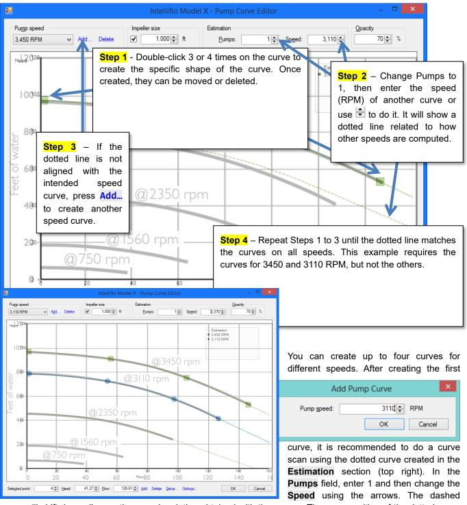
curve will shift depending on the speed variation obtained with the arrows. The superposition of the dotted curve with the different curves in the graph will determine whether the addition of a second curve is required. If this is the case, the **Pump speed** section, click the **Add** ... and enter the RPM for which the second curve must be created and use the same steps as before to create the new curve.
