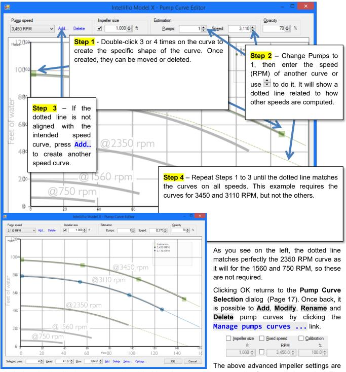
used when the impeller is worn or not the original impeller or an adjustment to the flow results is required. The setting compensates for the impeller size, speed or calibration. These adjustments will only affect the system curve and not the pump curve loaded into the instrument.
