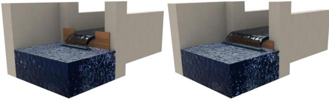
The accuracy of rectangular weirs, with or without contractions, is usually between 1 to 4% of the flow coefficient when all conditions are met.
