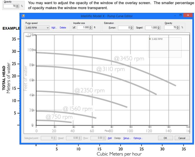
When overlapping the windows, be sure to use identical scales and adjust the window size for a perfect overlay of the graph of the pump curve document. Place the origin of the axes over each other to start and stretch the top right sides of the **Pump Curve Editor**.
