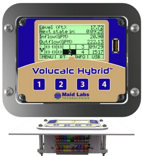
Once the instrument is fixed, connecters must be removed in order to connect wires to them. If needed, removing the instrument from the panel takes only a minute or so.
