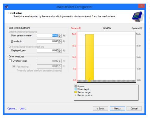
If a level sensor is configured a the **Inputs and outputs page**, the Level setup dialog will be displayed and a graph will show the range of the sensor with other options like the possibility to record sewage sewer overflow events including volume lost during the event.
