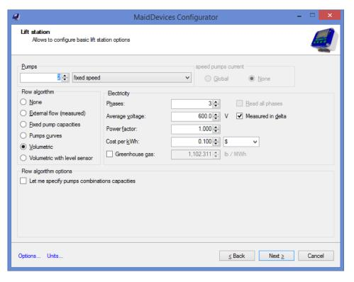
Flow algorithm selects how the flow is calculated. If the instrument is not used for flow calculation, select None.
