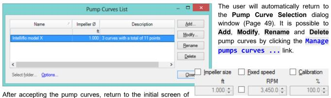
the **Pump Curves Selection**. These are advanced impeller settings and only used when the impeller may be worn or not the original impeller do to maintenance requirements. The setting will compensate for the impeller size, speed or calibration. These adjustments will only affect the system curve and not the pump curve you may
