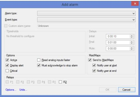
**Must acknowledge to stop alarm** is used to display the alarme on the device and require a used to acknowledge it or it will always stays on top.
