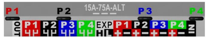
The analog input Level is configurable in the I/O column. The choices are 4-20 mA, 0-5V, 0-10V and 0-24V. The choice of sensors include: Sick 1.3 m, Sick 6m, Custom level or
