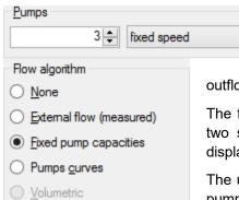
In the **Lift station** dialog window, when all pumps are constant speed, the flow algorithm will use the preset pump capacities. Based on run times for each pump, the total volumes per pump and total volumes pumped (all pumps) will be calculated as
